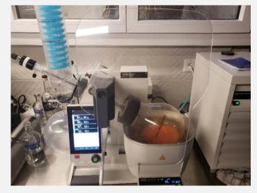
During the second day of my training, I worked in the laboratory with Dirk Hany who showed me different ways of infusing liquids. He introduced me in the process of work with Rotavap – high pressure distillation, where under vacuum is created a high pressure which allows liquids get to their boiling point at much lower level. This method is really good for clarifying spirits after they have been infused with ingredients with a different structure.
